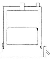
device is useful for small laboratory steam-ovens, since the base can be readily freed from scale, and renewed if necessary. It is, however, particularly valuable for larger combined ovens and stills. For these, the top of the oven is fixed rigidly to a stand, the base being supported on two cranked rods, to which handles are attached, by the turning of which the base may be instantly lowered and removed for cleaning. In ovens which are fitted with a reflux condenser and water gauge and are
